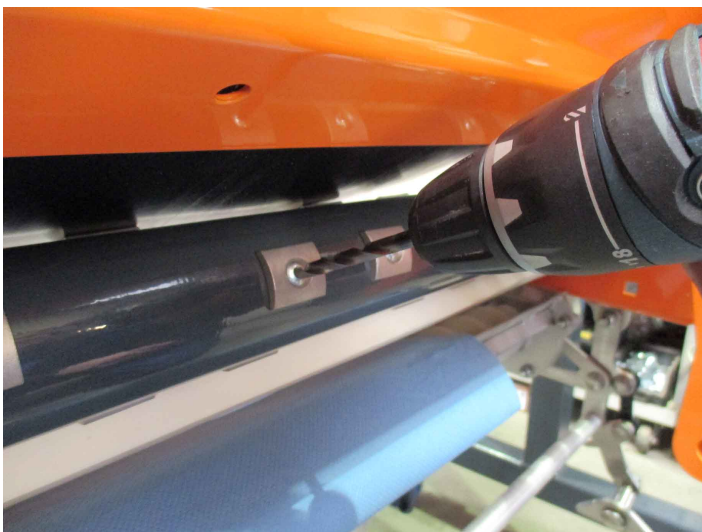
Illustration 15: Drill out the rivets.
