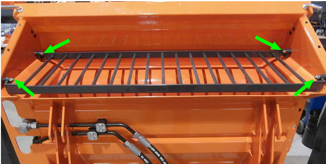
Illustration 9: Dismantle the protective grille.
