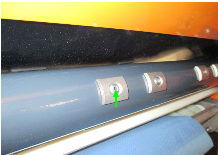
Illustration 14: Pierce the pin for drill centring.
