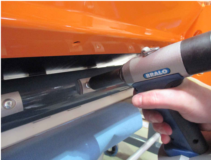
Illustration 17: Rivet the new cams.
