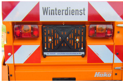
Illustration 3: Duplicate numberplate mounting
